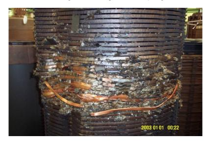
Figure 2. Catastrophic Failure of a Transformer (Image Source: OilRegeneration.com)
