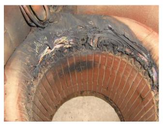
Figure 1. Defective Stator Winding of a Welding Alternator (Image Source: WindingPhotos)
