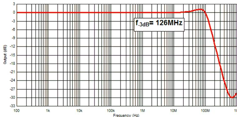
Figure 3. Closed-loop Bandwidth of a Buffer
