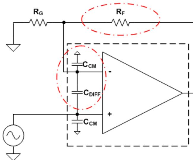
**Figure 1. Op-amp Model Showing Input Common-mode and Differential Capacitance**
