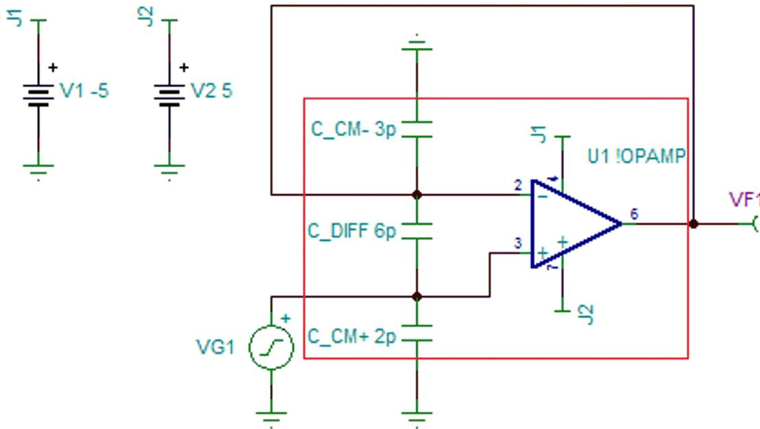
Figure 2. TINA-TI Software Schematic of an Op-amp Buffer
