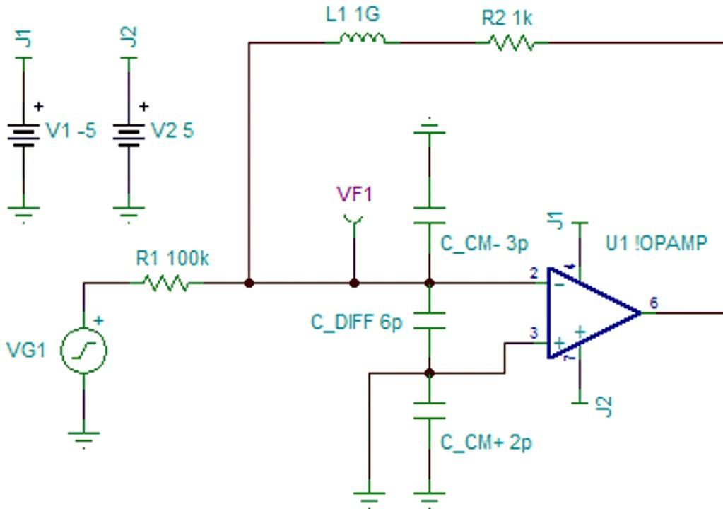
Figure 8. TINA-TI Software Schematic  $C_{DIFF}$
