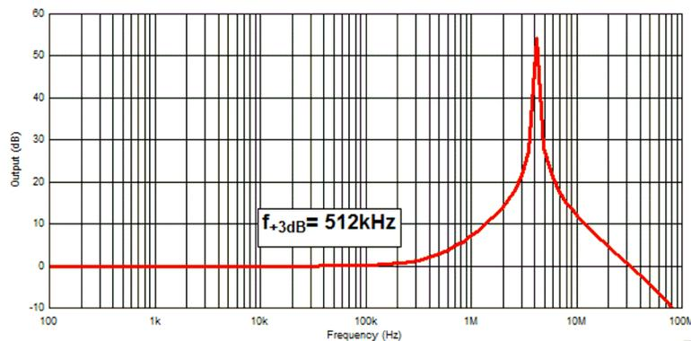
Figure 7. Simulated Response for  $C_{CM-}$  Extraction
