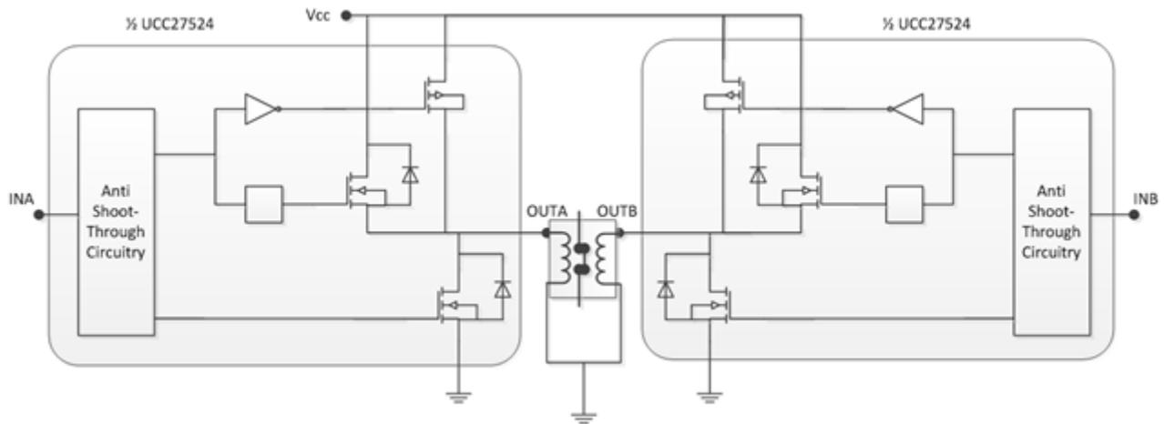
**Figure 3. Dual-coil Configuration for a Latching Relay in E-metering Applications**
