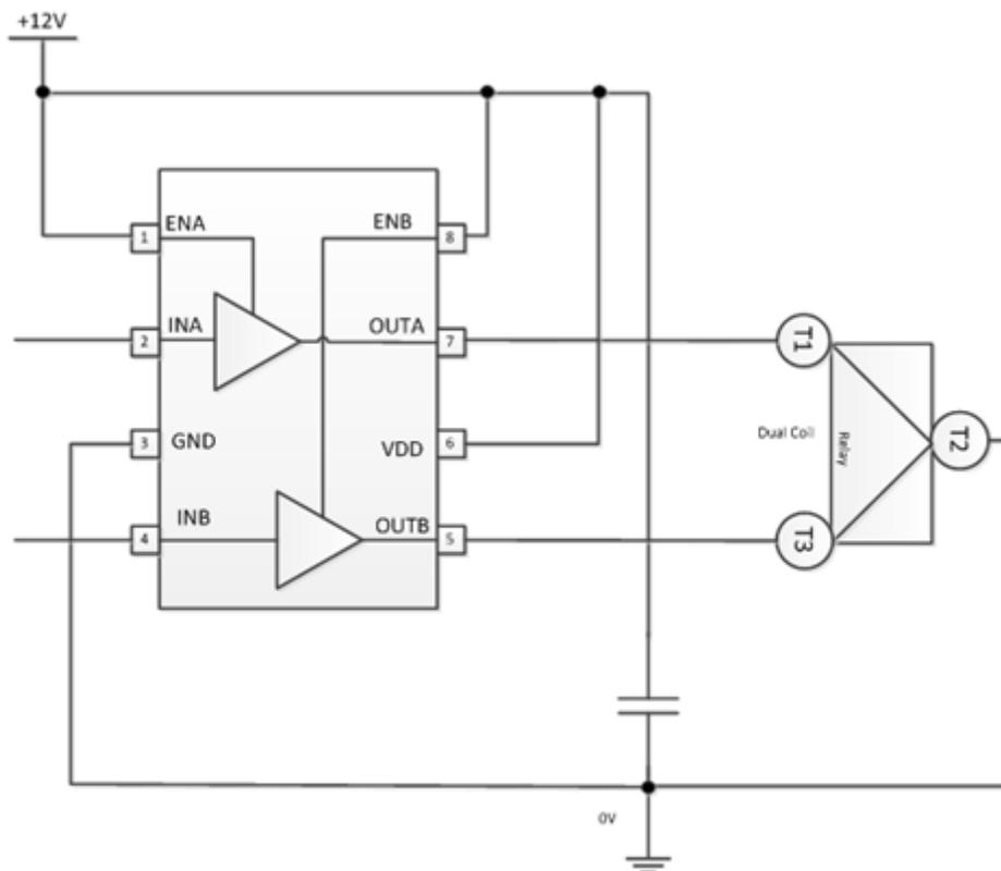
Figure 2. Simplified Schematic for Dual Coil Configuration Drive Circuit
