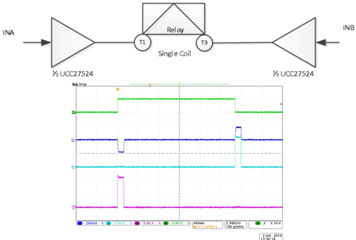
Figure 6. Simplified Schematic for Single Coil Configuration Drive Circuit
