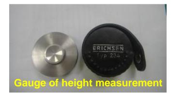
Flux/paste dipping depth was measured by using height gauge shown in below picture.
