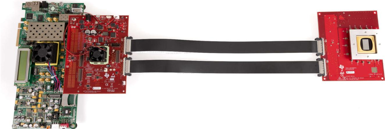
Figure 2-6. Fully Assembled DLPLCRC964EVM with AMD EVM
