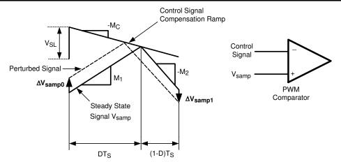
図 6-4. Compensation Ramp Avoids Subharmonic Oscillation
