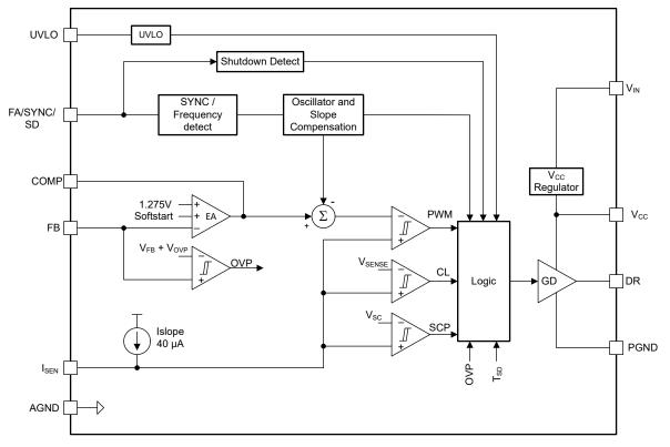
図 6-2. LM3481-Q1 Simplified Functional Block Diagram
