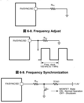
図 6-10. Shutdown Operation in Frequency Adjust Mode
