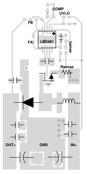
図 7-10. Typical Layout for a Boost Converter
