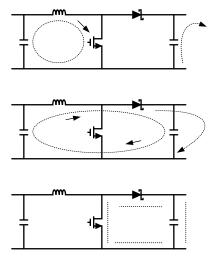
図 7-9. Current Flow in a Boost Application
