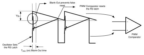
図 6-1. Basic Operation of the PWM Comparator
