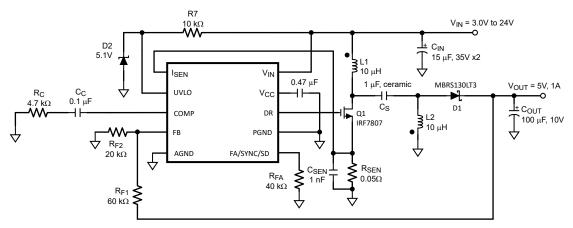
☑ 7-7. Typical SEPIC Converter using LM3481-Q1
