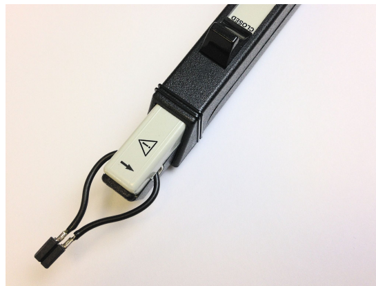
Figure 21. Combination of Current Probe With Self-Made Adapter for Primary Side Current Measurement
