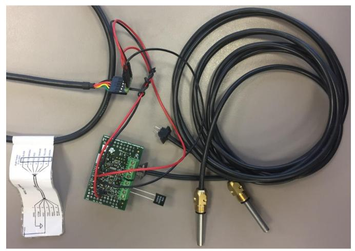
図 5. High-Precision Resistor and Two 2-Wire PT1000 (USB-to-UART Cable to PC)
