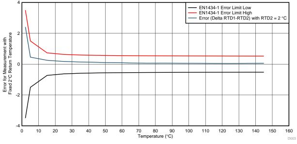
図 9. Absolute Temperature Accuracy of Two PT500 Sensors in 2-Wire Configuration
