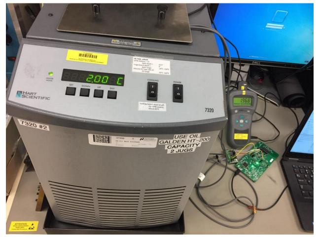
図 7. Test Setup for TIDA-01526 With 7320 Oil Bath and HART1521 Calibrated Thermometer
