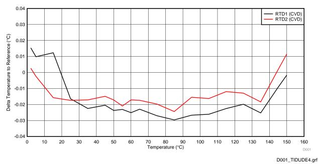
☑ 10. Absolute Temperature Accuracy of Two PT1000 Sensors in 4-Wire Configuration
