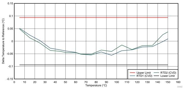
図 8. Absolute Temperature Accuracy of Two PT500 Sensors in 2-Wire Configuration
