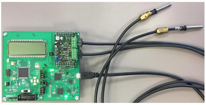
☑ 6. MSP430FR6047EVM With TIDA-01526 Mounted and Two 2-Wire PT1000 Sensors and the USB Connection to PC (UART Back-Channel Support)
