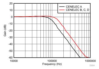
図 30. TX Filter Gain vs Frequency
