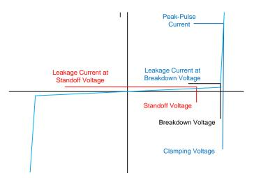
図 24. Typical Bidirectional TVS I/V Characteristics
