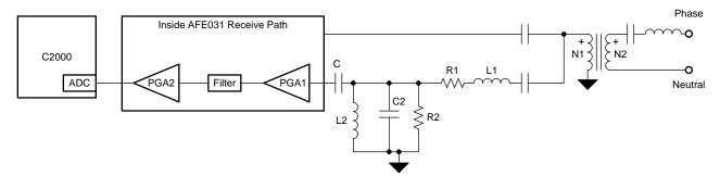
図 39. AFE031 Receive Path Interfaced With C2000™ ADC
