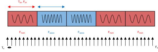
図 42. Received FSK Signal
