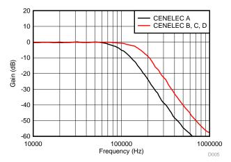
図 41. RX Filter Gain vs Frequency
