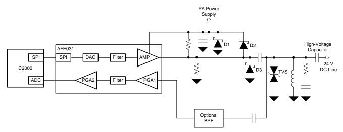
図 17. Coupling Circuit for a DC Line
