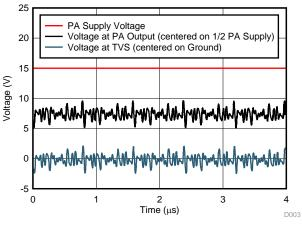
図 25. Typical Signal at TVS
