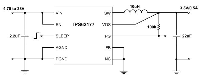
図 4. Typical Application Schematic of TPS62177
