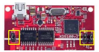
図 13. F28379D Jumper Configuration
