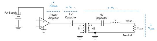
図 27. Typical Line Coupling Circuit
