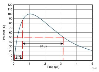
図 22. Typical 8/20-µs Pulse for MOV and TVS Performance Specification
