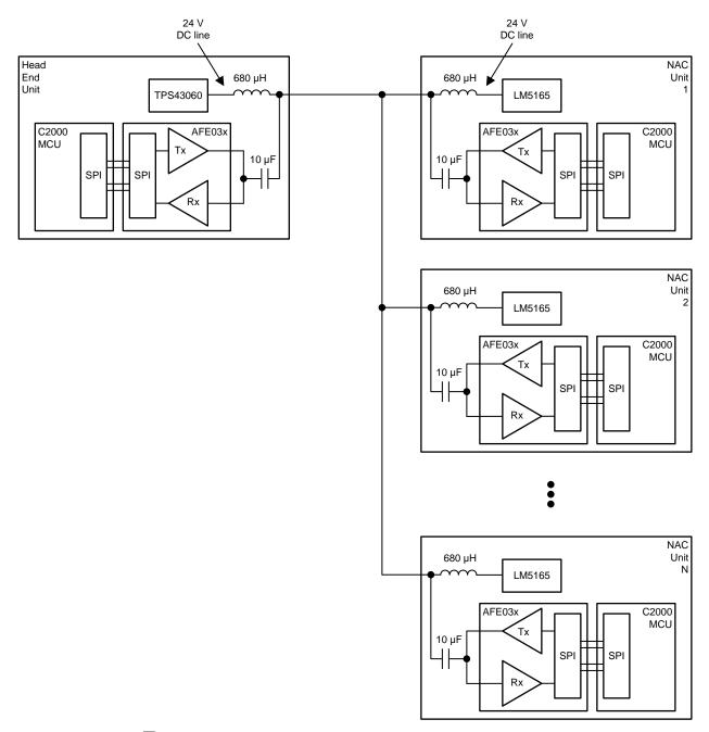
図 18. Example of Multiple PLC Modules Coupled to a DC Line
