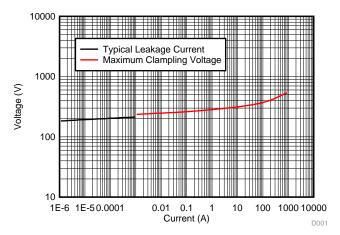
図 21. Typical MOV I/V Characteristic
