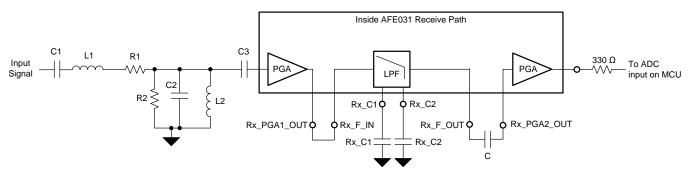
図 40. External Filtering for the AFE031 Receive Path
