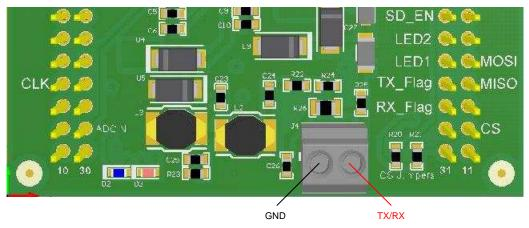
図 12. BOOSTXL-AFE031 Terminal Block Connections
