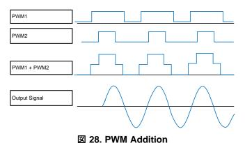
☑ 29 shows the path of the PWM signals. The PWM signals go into the low-pass filter internal to the AFE030/AFE031 device, and are added together to create the above PWM1+PWM2 waveform. ☑ 30 shows the gains witnessed at certain frequencies at the output of the internal TX low-pass filter.
