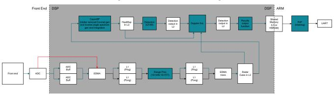
As shown in 🗵 5, the implementation of the Automated Doors example in the signal-processing chain consists of the following blocks implemented as DSP code executing on the C674x core in the IWR6843:
