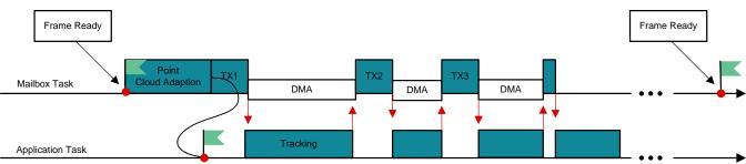
図 6. High-Level Processing Task Model
