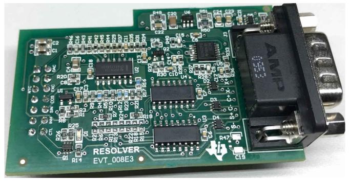
図 3-18. Resolver Analog Front End Module
