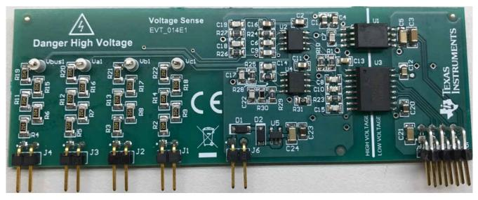
図 3-25. Inverter Voltage Sense Board
