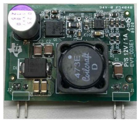
図 3-13. Vbat to 12-V/1-A Power Supply Module
