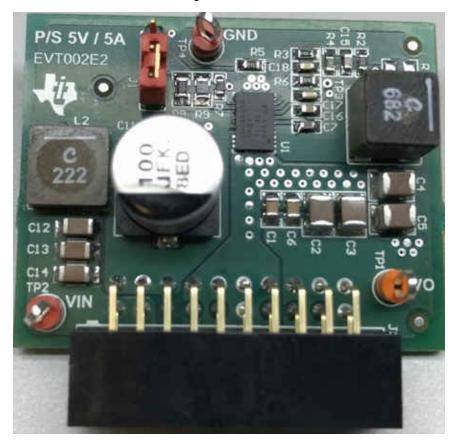
図 3-12. Vbat to 5V/ 5A power supply module
