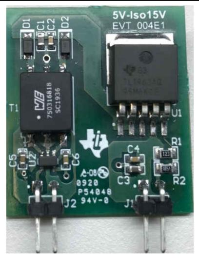
図 3-14. 5-V to 15-V/0.5-A power supply module
