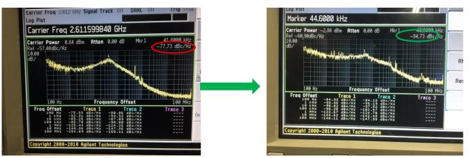
Figure 8. Phase Noise Improved by Using Good PSRR for the PLL VCO Power Supply
