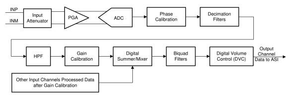
Figure 1. PCM6xx0 Channel Signal Chain Processing Flow Chart
