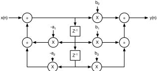
Figure 2. Direct Form II Biquad Filter
