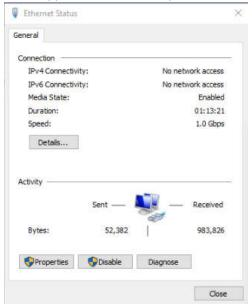
Figure A-4. Opening the Properties Tab for the Ethernet Connection
