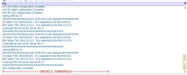
Figure 4-16. AFE Configuration Complete Showing Link Up for the Device's JESD RX
