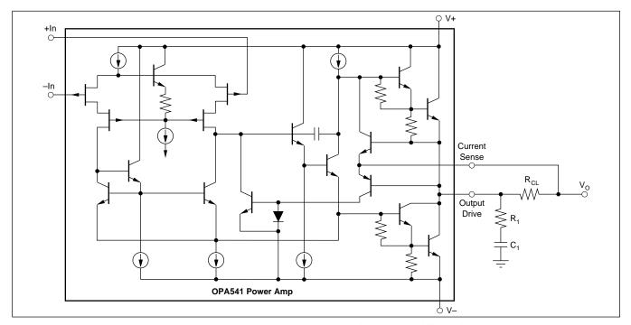
FIGURE 1. An R<sub>1</sub>, C<sub>1</sub> network can be added to the OPA541 output to improve stability during current limit.
