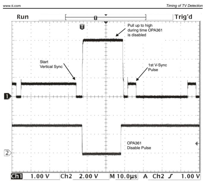
Figure 10. Detailed View of Disable and Enable Timing for OPA361
