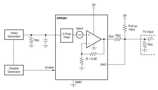
Figure 6. Evaluation System for the TV Detection Concept
