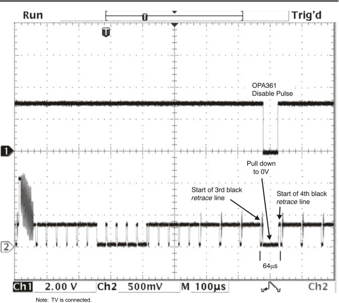
Figure 14. TV Detection During Fourth Black Retrace Line
