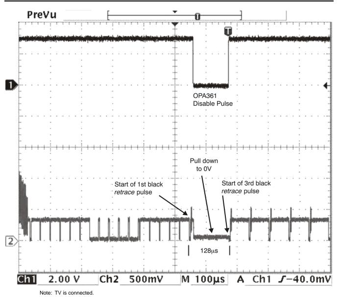
Figure 15. TV Detection During First and Second Black Retrace Line
