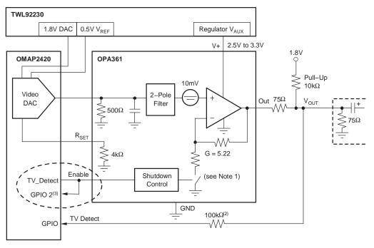
(1) Closed when enabled during normal operation; open when shut down.
