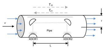
Figure 1. TOF Measurement in an Ultrasonic Flow Meter
