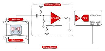
Figure 2. Typical Receive Path Circuit Using the OPA838
