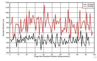
Figure 3. 200-kHz Single-Shot Standard Deviation (STD) OPA838 vs OPA836
