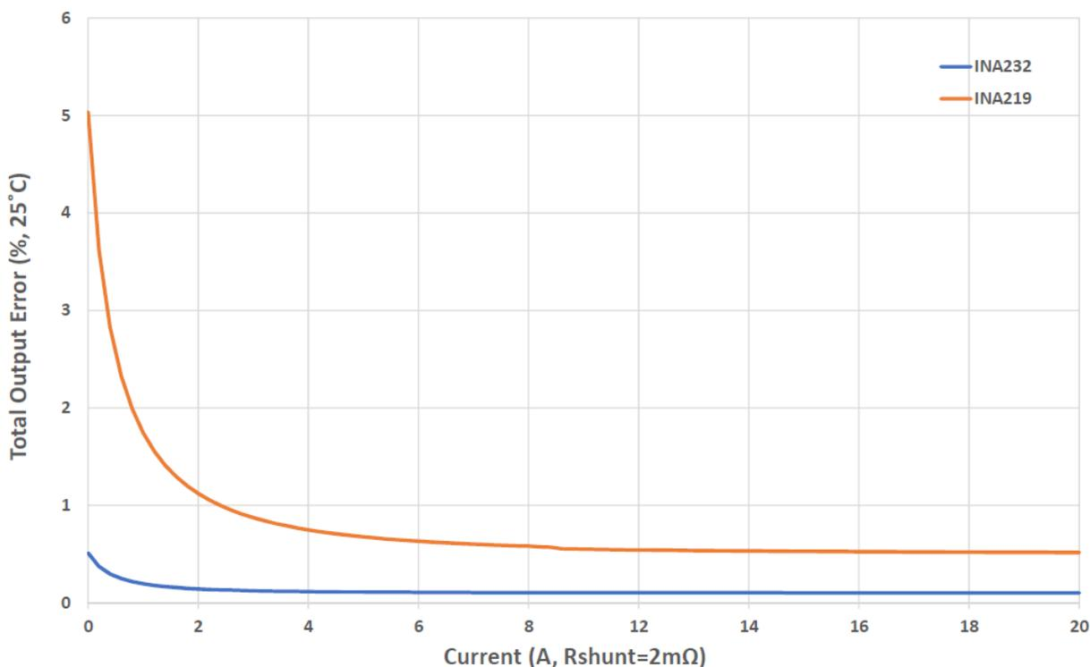
Figure 2-2. Total Output Error
