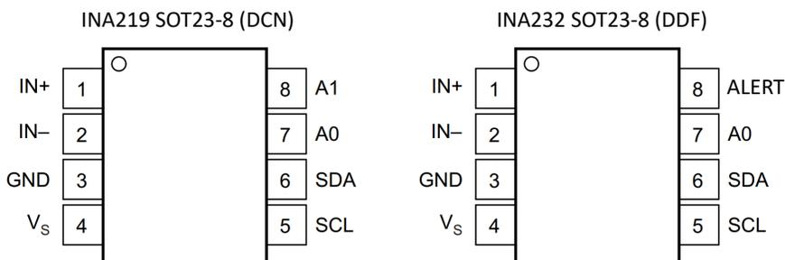
**Figure 2-1. Package and Pinout**
