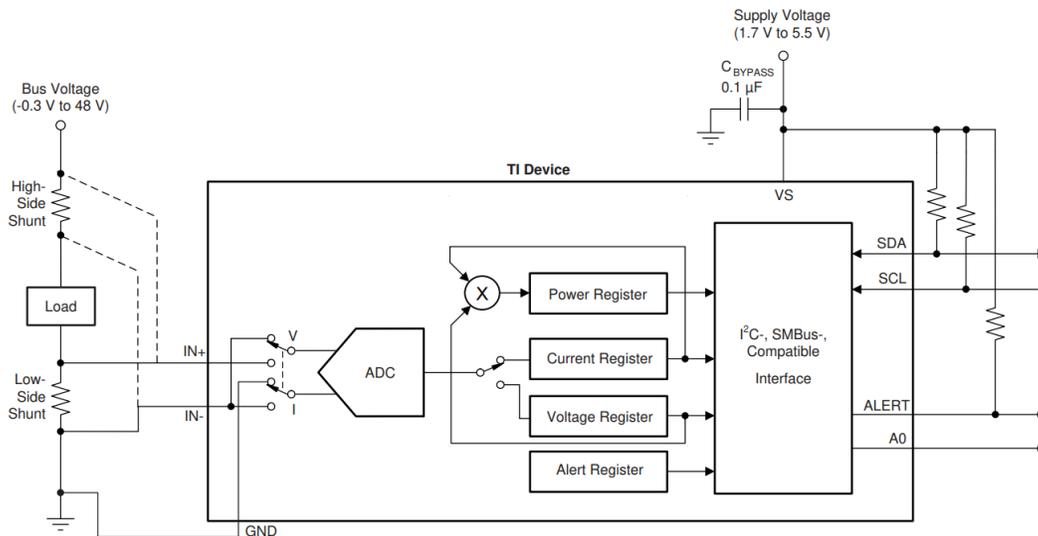
**Figure 1-1. Block Diagram of a Digital Power Monitor**
