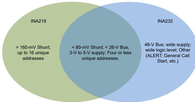
**Figure 3-1. Key Features and Supported Design Parameters**
