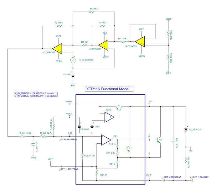
Figure 3-1. TINA TI Schematic and Simulation for 0-lbs Input
