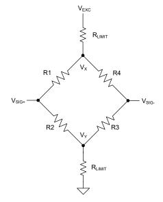
Figure 2-3. Current Limited Wheatstone Bridge Configuration
