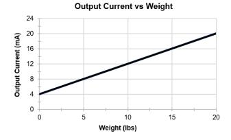
Figure 1-1. Measured Output Current vs Weight Transfer Function
