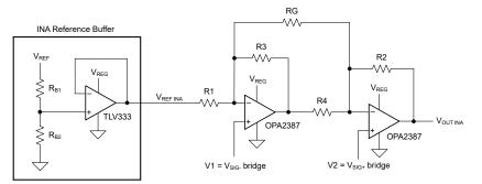
Figure 2-4. Discrete 2-Amp INA Configuration
