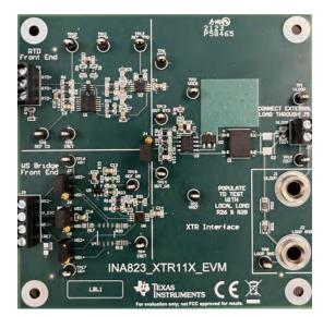
Figure 1-2. Wheatstone Bridge to 4-20-mA Current Loop Transmitter PCB Design
