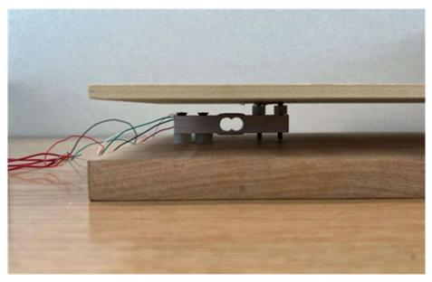
Figure 8-2. Mechanical Setup for Load Cell
