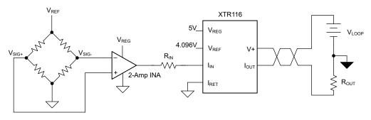
Figure 2-1. Simplified Bridge Amplification to 4-20-mA Circuit
