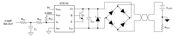
Figure 2-5. Surrounding Circuitry for Current Loop Transmitter
