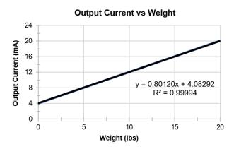
Figure 5-1. Measured Output Current vs Weight Transfer Function
