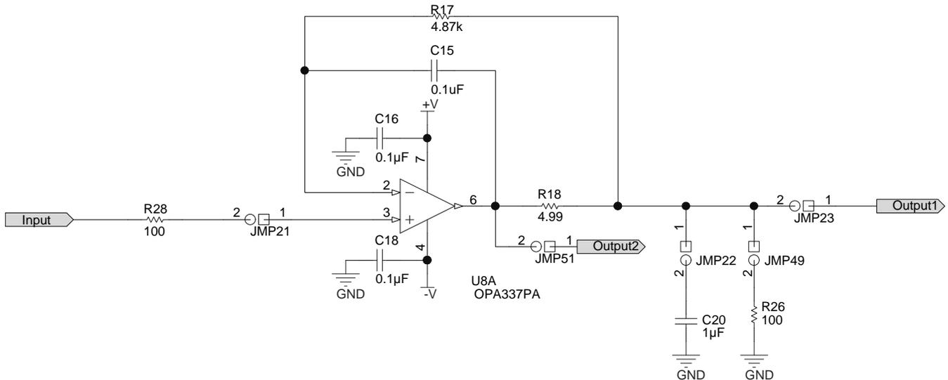
Figure 13. Circuit 6: Riso Dual-Feedback Stability Circuit
