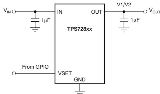
Figure 3. TPS728xx Application Circuit
