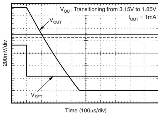
Figure 5. Typical Voltage Transition Waveform on VSET Toggle from 1→0
