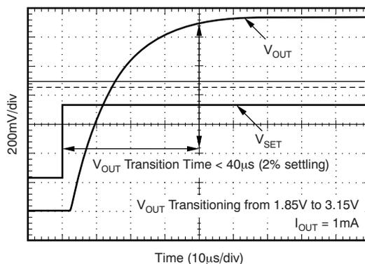
Figure 4. Typical Voltage Transition Waveform on VSET Toggle from 0→1
