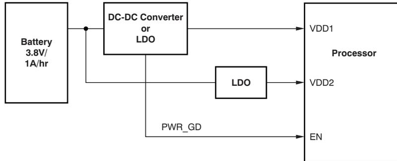
Figure 1. Typical Power Management Implementation for an Application Processor in a Mobile Phone
