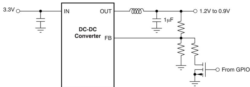
Figure 2. DVS Implementation on a DC-DC Converter with External Components
