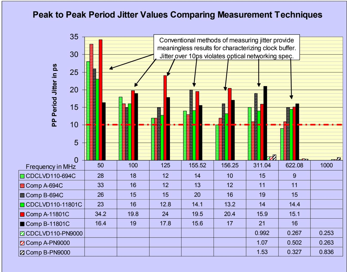
**Figure 4. Peak-to-Peak Period Jitter Compared Among Three Different Test Setups**
