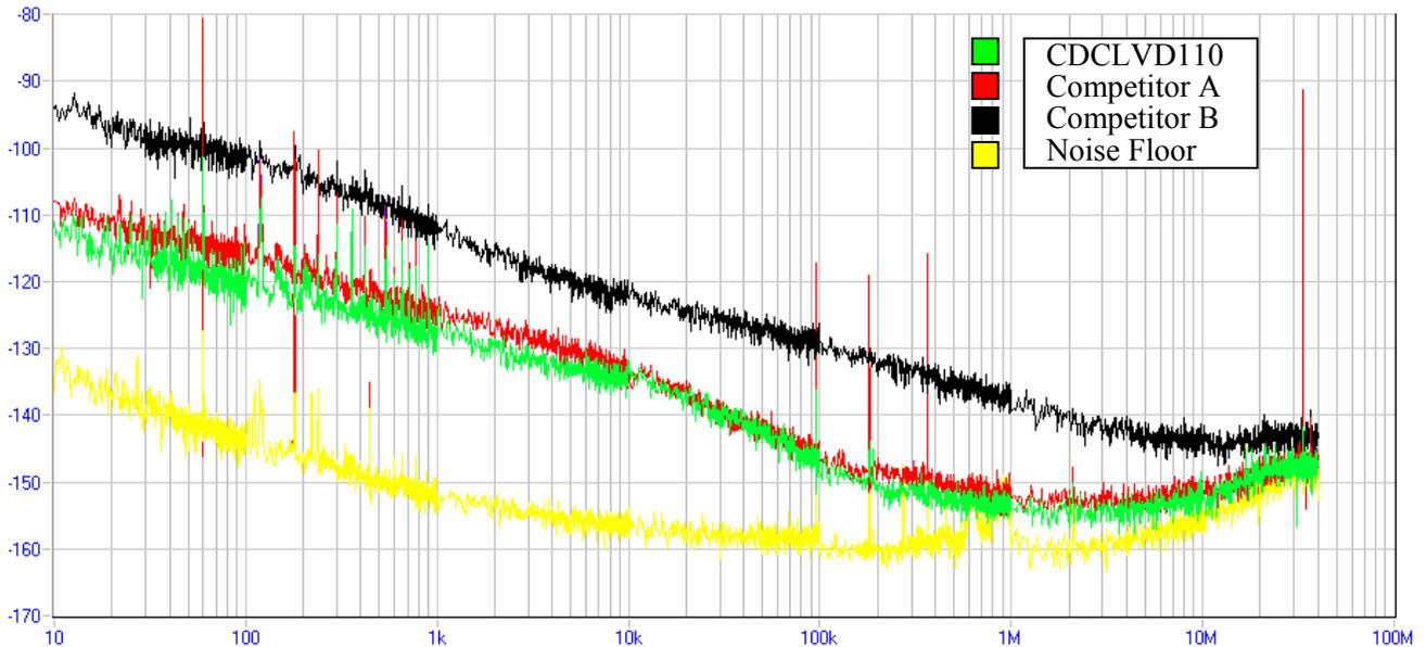
**Figure 6. Phase Noise Comparison at 622.08 MHz**
