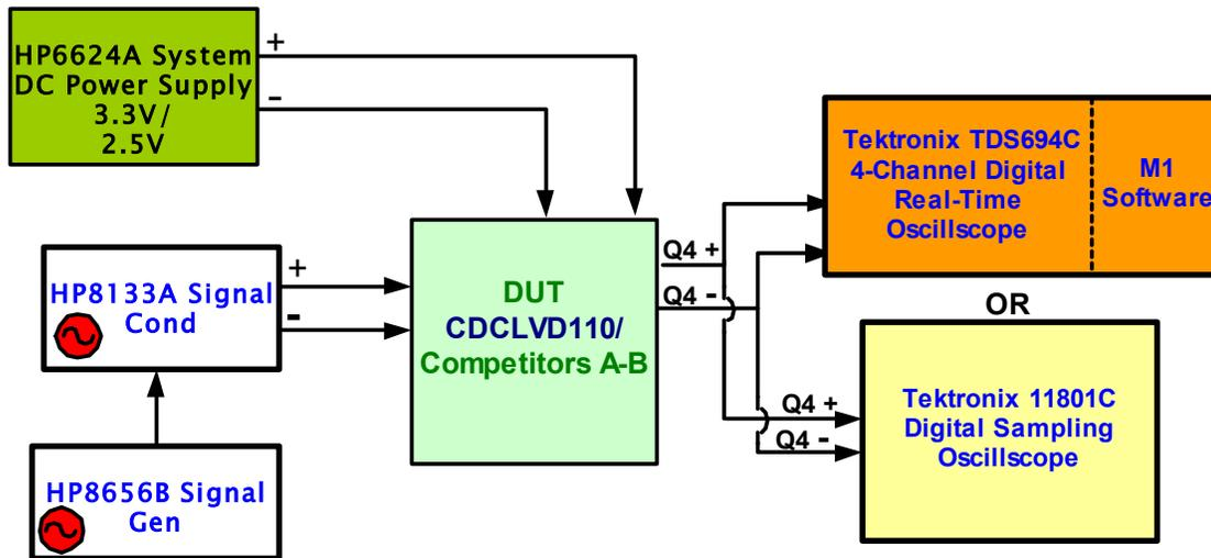
**Figure 2. Test Setup for Jitter Measurements Taken From Tektronix TDS694C and 11801C**
