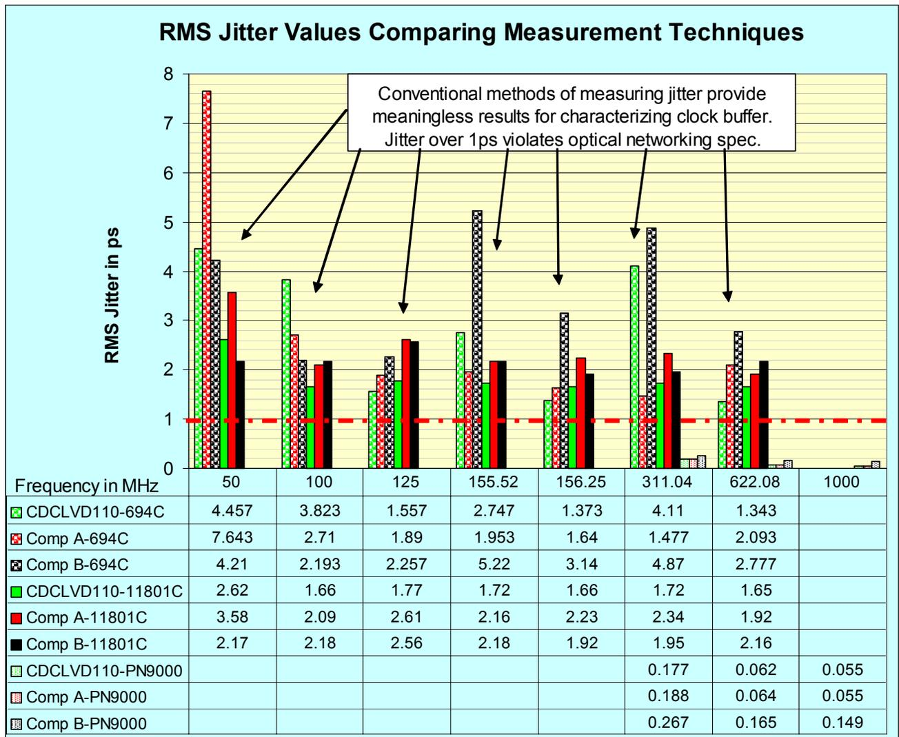
**Figure 3. RMS Jitter Values Compared Among Three Different Test Setups**
