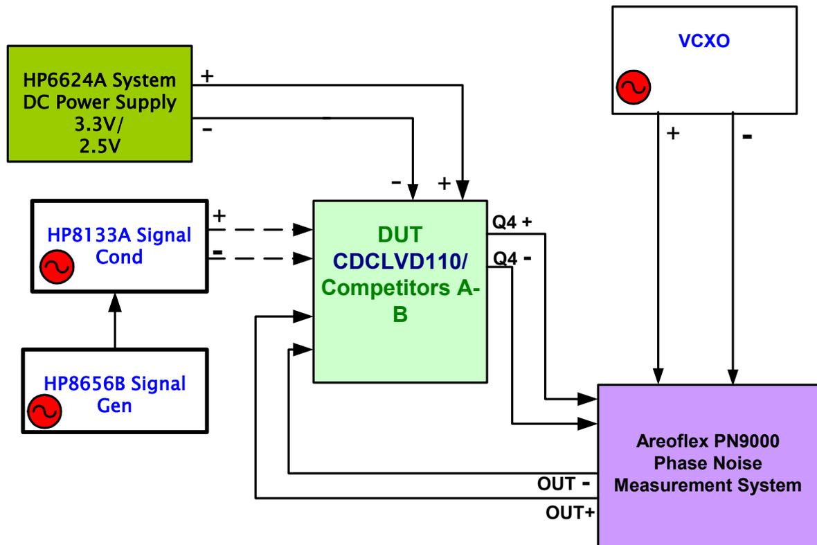
**Figure 1. Test Setup for Phase Jitter Measurements Taken From AeroFlex PN9000**
