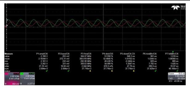
Figure 3-11. TXV Outputs (15 pF 1.8 V to 3.6 V Up Translation at 300 MHz, 25°C)
