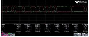
Figure 3-5. TXV Outputs (10 pF 1.8 V to 3.3 V Up Translation at 125 MHz, 25°C)
