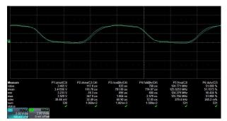
Figure 3-2. Competitor Outputs (5 pF 1.8 V to 3.3 V Up Translation at 125 MHz, 25°C)
