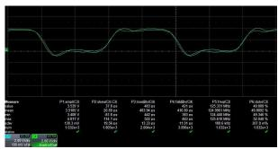
Figure 3-1. TXV Outputs (5 pF 1.8 V to 3.3 V Up Translation at 125 MHz, 25°C)
