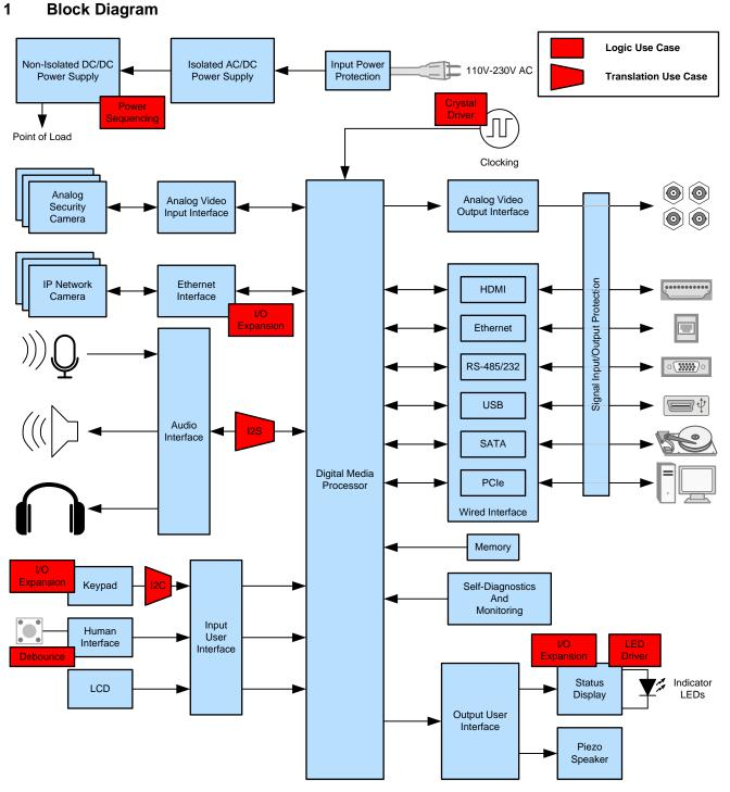
Figure 1. Simplified Block Diagram for Digital Video Recorder
