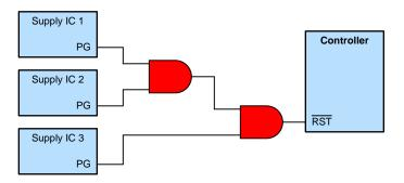
Figure 4. Using Logic to Combine Multiple Power-good Signals.
