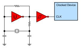
Figure 6. Using an Unbuffered Inverter and Schmitt-trigger Inverter to Generate a Clock Signal From a Crystal Oscillator.
