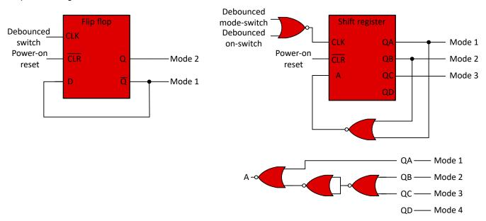
Figure 2. Separate Inputs for Mode Control and Device Enable
