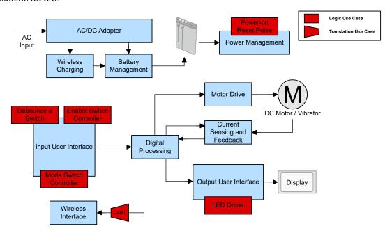
Figure 1. Simplified Block Diagram for Personal Care Electronics
