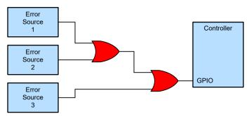
**Example Block Diagram for Combining Three Error Sources Into One Error Signal Using OR Gates**
