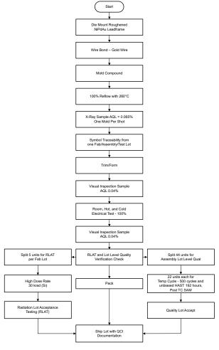
Figure 2-1. SN54SC6T14-SEP Space Enhanced Plastic Production Flow Chart
