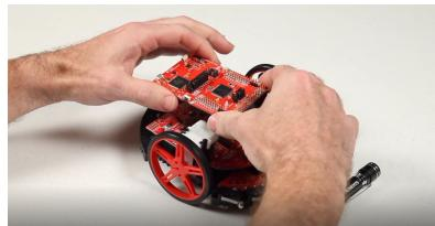
Figure 1 Dis-assembly of TI-LaunchPad from the robot
