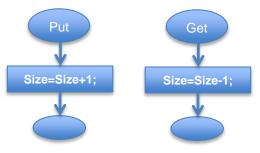
In summary, the UART driver will use interrupt synchronization with FIFO queues. This buffered approach will decouple the production of data from the consumption of data. For example, the main program can generate data to print, and put it into the FIFO queue. When the transmit UART hardware is idle, the ISR can get from the FIFO and write the data to the hardware. Buffering data in this matter is an efficient and effective mechanism for complex systems.
