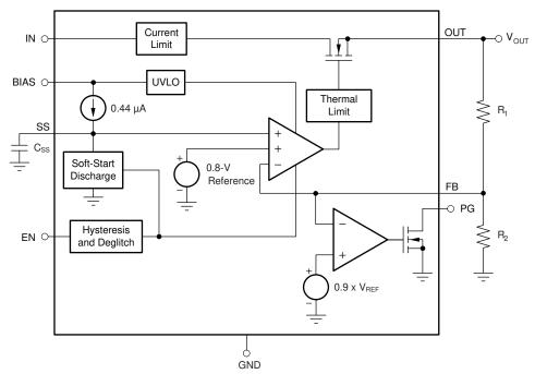
Figure 1-1. Functional Block Diagram
