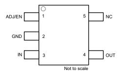
Figure 4-1. Pin Diagram (DBV) Package
