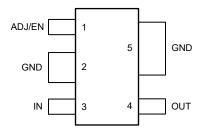
Figure 4-2. Pin Diagram (DYB Package)
