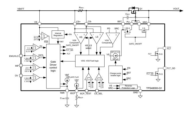
Figure 1-1. Functional Block Diagram
