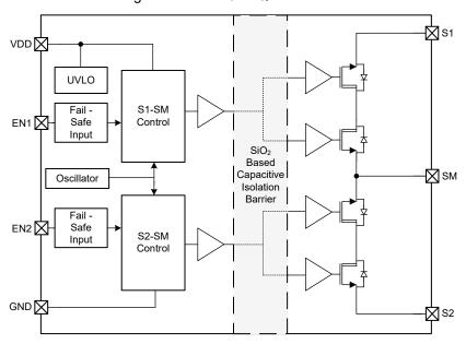
Figure 1-1. TPSI2072-Q1 Functional Block Diagram
