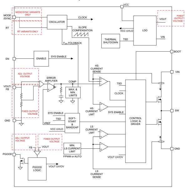
Figure 1-1. Functional Block Diagram
