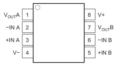
Figure 4-2. Pin Diagram (SOIC Package)
