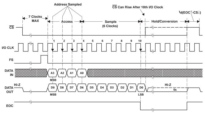
NOTES: D. The falling edge of FS has to appear within 7 I/O clock cycles from the falling edge of  $\overline{CS}$ .
