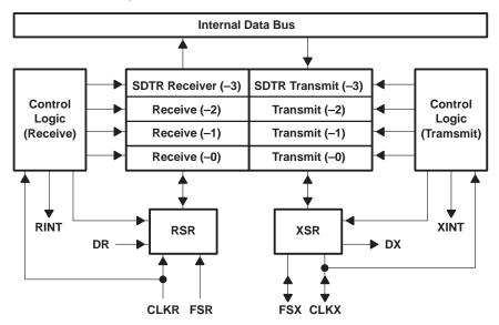
Figure 8. Synchronous Serial Port Block Diagram
