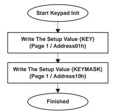
Figure 4. TSC2301 Keypad Driver Initialization—InitTSC2301Key()
