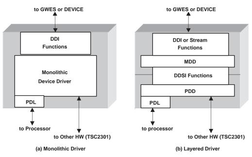
Figure 2. Monolithic and Layered TSC2301 Driver
