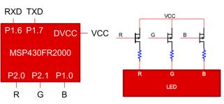
Figure 1. RGB LED Controller Block Diagram
