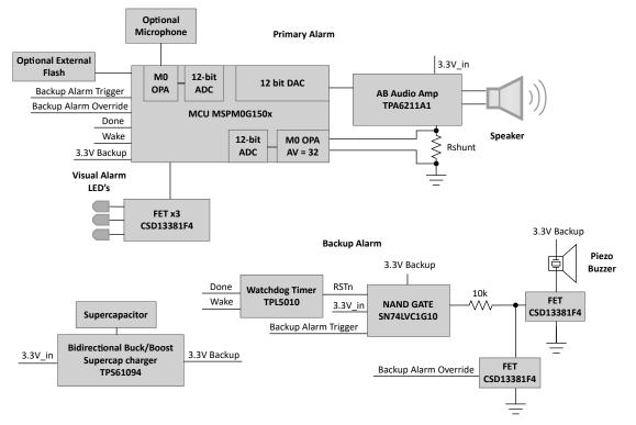
Figure 1. Design Block Diagram
