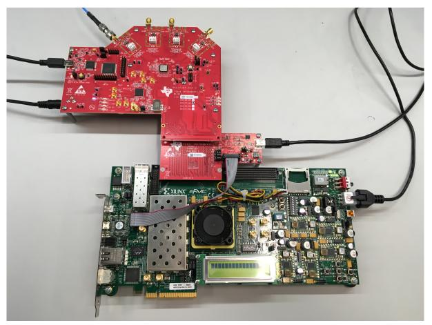
Figure 7. DAC38J84EVM GUI Setup Example
