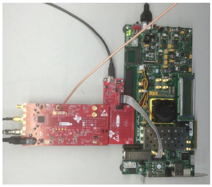
Figure 13. ADC32RF45EVM, TSW14J10EVM and VC707 Board
