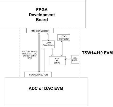
Figure 2. TSW14J10 EVM Block Diagram
