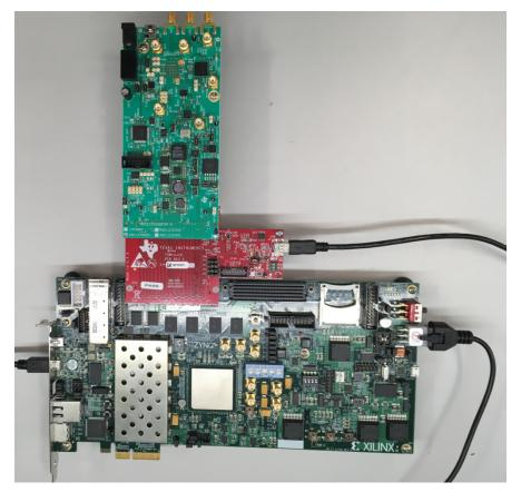
Figure 24. ADC12J4000EVM, TSW14J10EVM and ZC706 board
