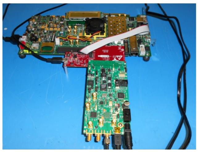
Figure 18. ADC12J4000EVM, TSW14J10EVM and VC707 Board
