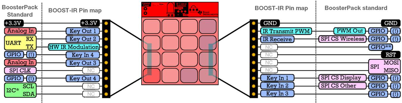
Figure 3. BoosterPack Pinout
