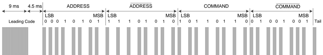
**Figure 12. Pulse Distance Protocol, Data Frame Format**
