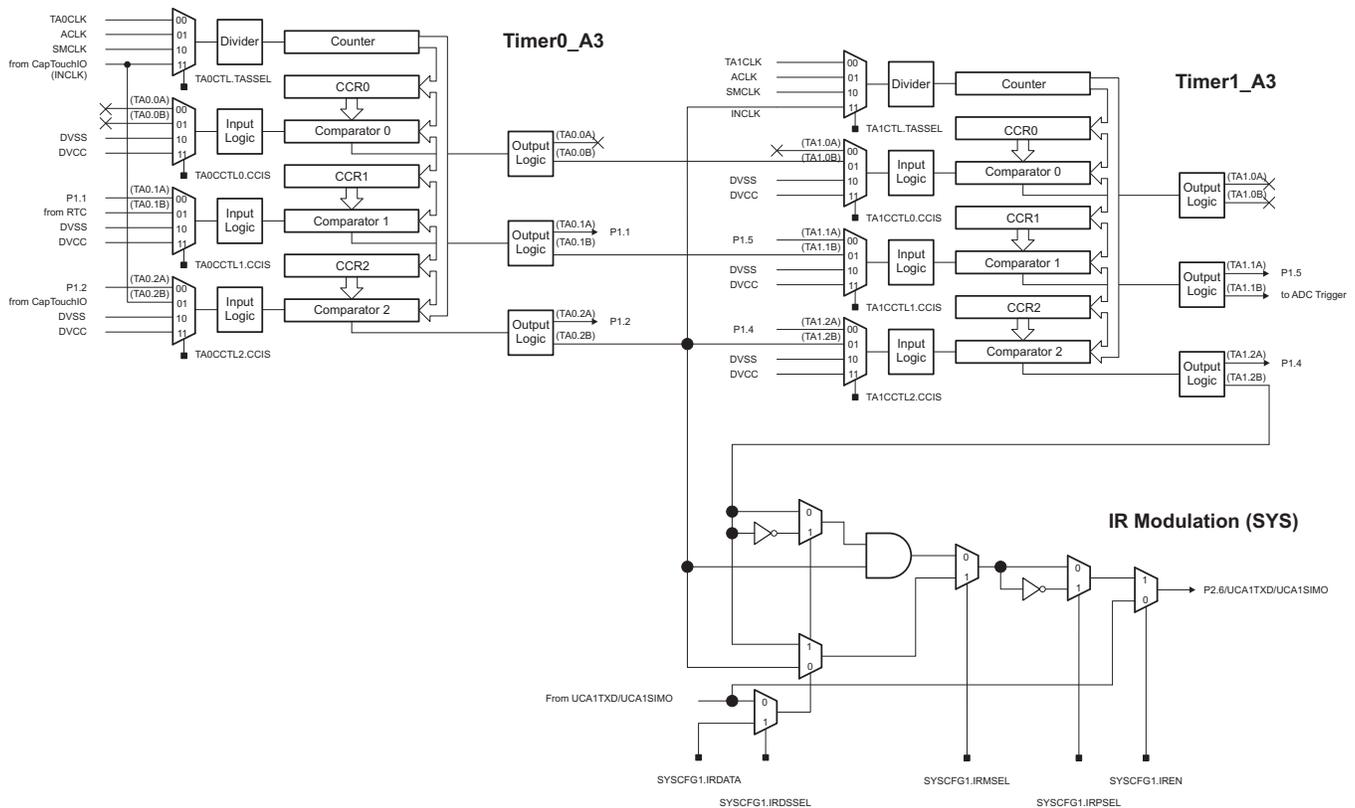
Figure 8. IR Modulation Logic Blocks in MSP430FR4133
