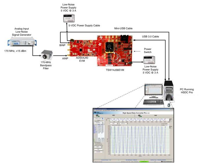
Figure 2. Quick Start Test Setup
