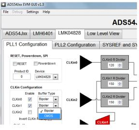
Figure 8. GUI CMOS Selection
