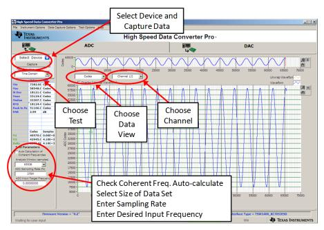
Figure 4. HSDC Pro GUI Main Panel
