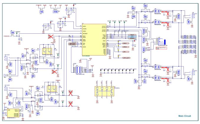
Figure 4-3. TAC5112 EVM Main DUT Schematic
