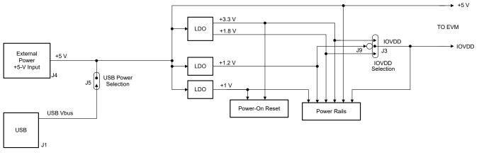
Figure 2-7. Power-Supply Distribution of the AC-MB
