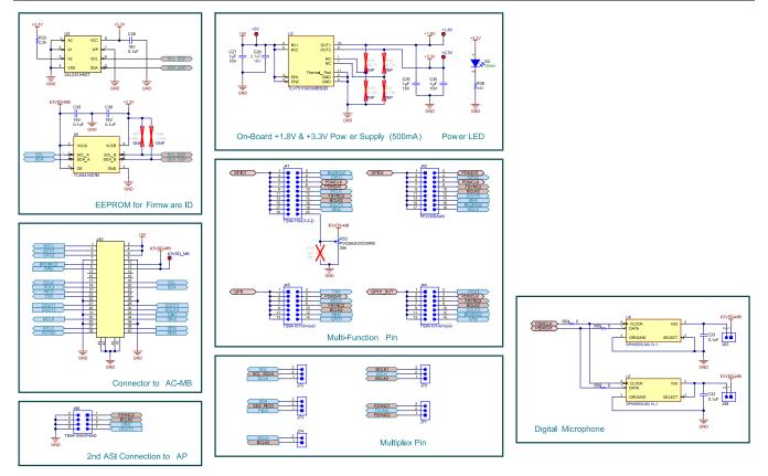
Figure 4-6. TAD5212 EVM Connectors and Supporting Circuitry Schematic
