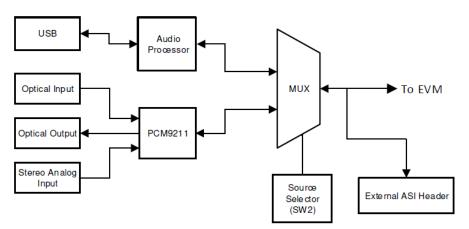
Figure 2-2. AC-MB Audio Interface Block Diagram
