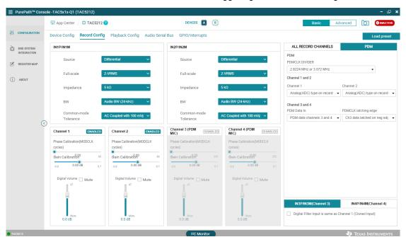
Figure 3-12. PDM Record Config Tab
