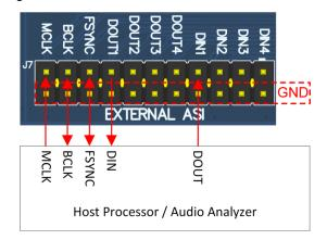
Figure 2-6. AC-MB Connection with External Audio Serial Interface
