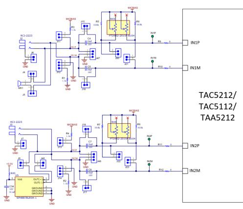
Figure 2-8. TAC5212 and TAC5112 EVM Input Architecture for Channel 1 and 2
