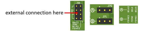
Figure 2-17. External Audio Serial Interface Connection
