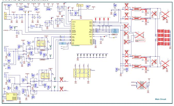
Figure 4-5. TAA5412-Q1 EVM Main DUT Schematic
