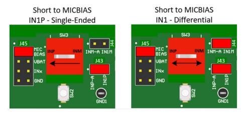
Figure 2-15. Short to MICBIAS Diagnostic Test Setup
