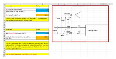
Figure 2-10. AC-Coupled External Resistor Calculator
