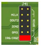
Figure 2-20. GPIO1 Configuration
