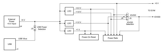
Figure 2-7. Power-Supply Distribution of the AC-MB
