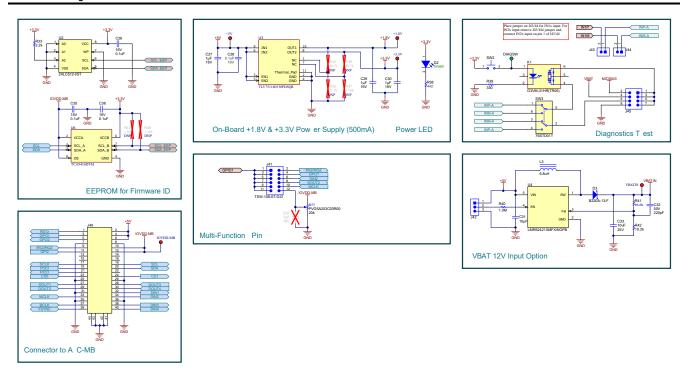
Figure 4-4. TAC5311-Q1 EVM Connectors and Supporting Circuitry Schematic
