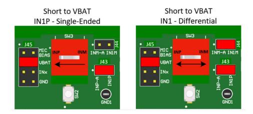
Figure 2-17. Short to VBAT Diagnostic Test Setup
