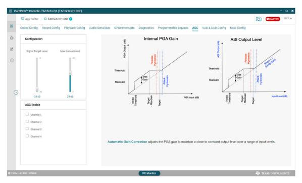
Figure 3-26. Automatic Gain Control (AGC) Tab
