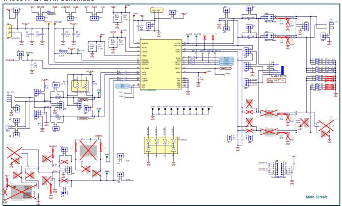
Figure 4-3. TAC5311-Q1 EVM Main DUT Schematic
