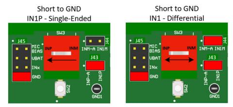
Figure 2-19. Short to Ground Diagnostic Test Setup
