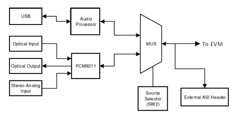
Figure 2-2. AC-MB Audio Interface Block Diagram
