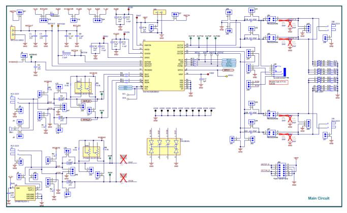
Figure 4-1. TAC5412-Q1 EVM Main DUT Schematic
