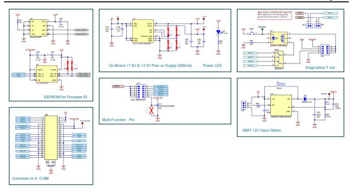
Figure 4-2. TAC5412-Q1 EVM Connectors and Supporting Circuitry Schematic
