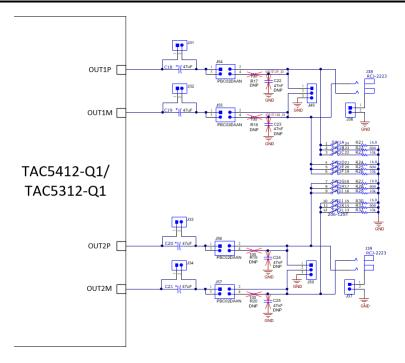
Figure 2-11. TAC5412-Q1/TAC5312-Q1 EVM Output Architecture for Channel 1 and 2
