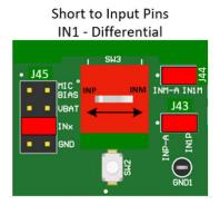
Figure 2-18. Short to Input Diagnostic Test Setup
