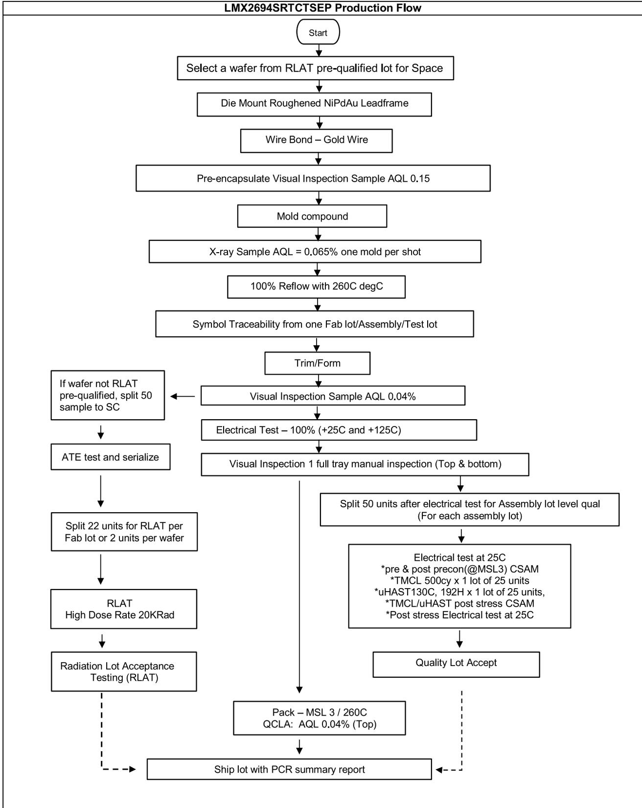
**Figure 2-1. Space Enhanced Plastic Production Flow**
