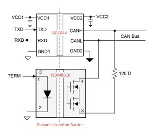
Example Isolated Software Controlled Termination Resistor Diagram Using an OptoMOS
