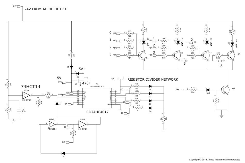
Figure 3. Proposed Solution to Control the Speed of the Fan by Toggling AC
