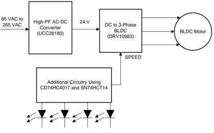
Figure 2. Modified Block Diagram
