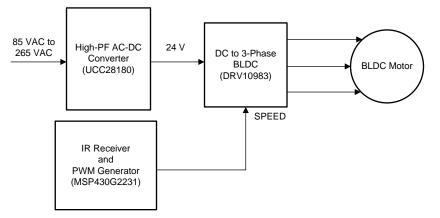
Figure 1. BLDC Ceiling Fan Demonstrated in TIDA-00652
