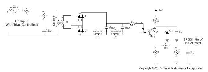
Figure 5. TRIAC-Based Control of AC Operated BLDC Fan
