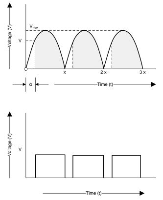
Figure 6. PWM Signal at Emitter of Optocoupler
