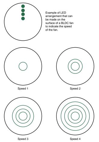
Figure 4. Probable LED Arrangement to Indicate the Speed of Fan
