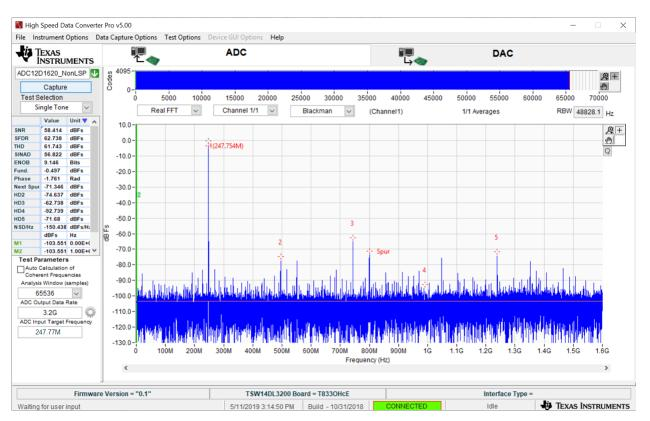
Figure 9. ADC12D1620QML-SP 3.2 GSPS Spectrum with LMH5401-SP Buffering 1.6 GHz Clock
