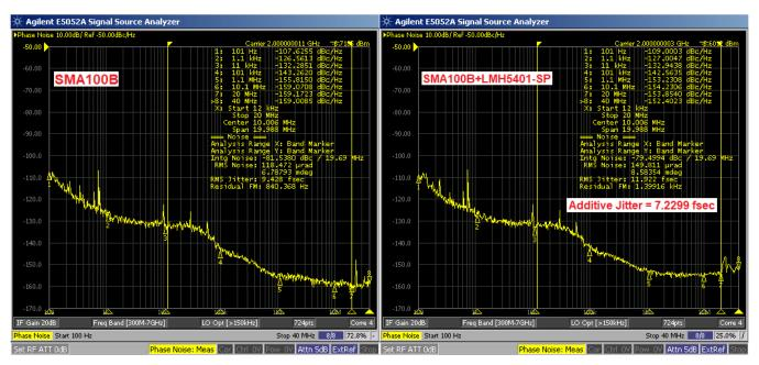
Figure 8. Phase Noise 2 GHz, Spurs-Include
