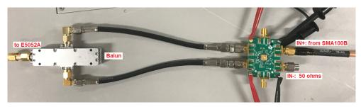
Figure 6. SMA100B + LMH5401-SP Phase Noise Setup
