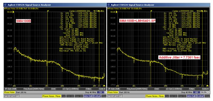
Figure 7. Phase Noise 2 GHz, Spurs-Omit
