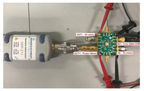
Figure 5. Determining Signal Source Power Levels
