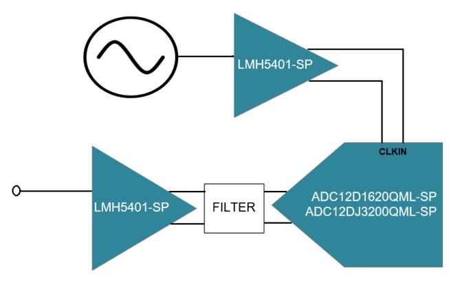
Figure 1. LMH5401-SP as Clock Buffer
