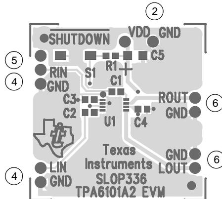
† Due to the very small size of the MSOP IC package, the standard part number TPA6101A2 is replaced with the code TIAJM.
