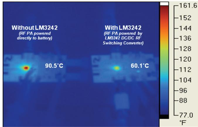
LM3242 reduces PA heat by 30°C at max RF power (28 dBm)
